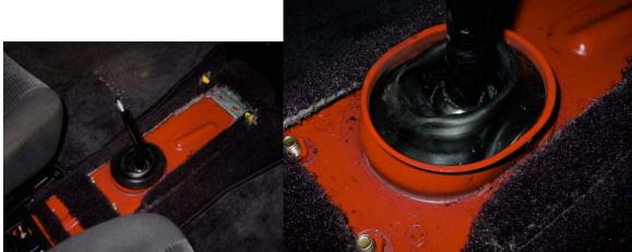
With the center console out of the way, pull back the weather seal.
