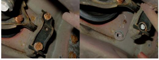
Up at the front, you need to remove the bolt that holds the front of the shifter rod with a 12mm box wrench. Energy suspension's shift stabilizer pictured.
