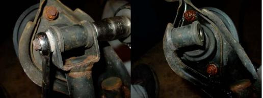
At this point, you will need to remove the two bolts that retain the shifter. It will be necessary to use vice grips to hold the top of the bolts.
