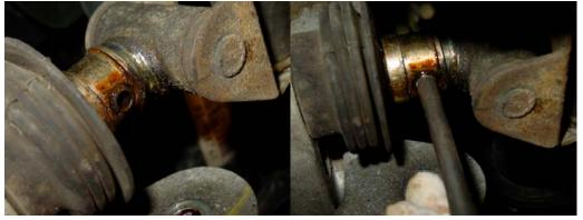
If you did not remove all of the shift linkage from the car, you will need to remove the bolt on the bottom of the shifter with 12mm wrenches. With the bolt out, you will need to remove the shifter and the rod on which the shifter pivots.
