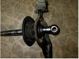
At this point, you need to slip the linkage and shifter back into the car (if you didn't remove all of it) or attach the other shift rod to the bottom of the shifter.
